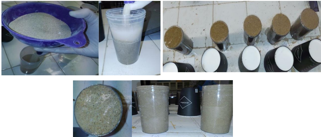
Figure 3. Preparation, pluviation by funnel and moulding of sand-MgO mix
